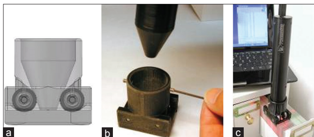
Figure 12: Slide tray attachment for ID reader. (a) Design. Photos of: (b) Slide drawer guide (“skateboard”) for ID reader; (c) Demonstration of reading the IDs of slides stored in a high capacity drawer
