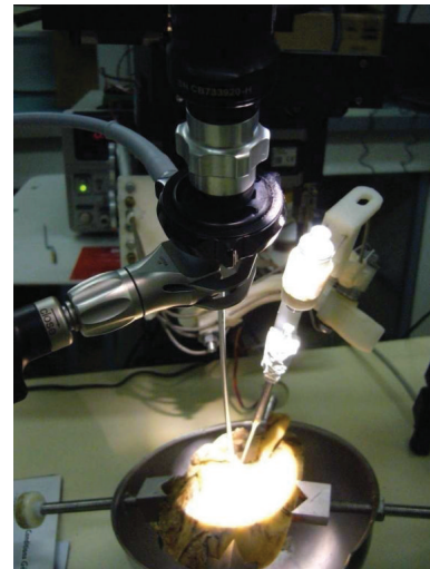
FIGURE 27: Simultaneous use of the robotic arm and a 4 mm endoscope in the external auditory canal.
