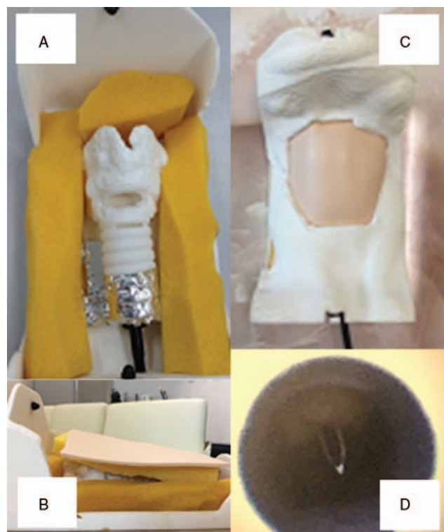
Figure 1. Simulator made with 3-dimensional (3D) printer. The frame of the simulator is based on data from 3-dimensional computed tomography scan data (local ethical committee approved). Face validity of the simulator was verified independently by 2 anesthesiologists. The simulator is equipped with an endoscope to observe inside the lumen of the simulated trachea.
