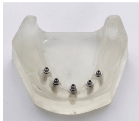
Fig. 1 Mandibular master model with five screw retained abutment in specific teeth positions.
