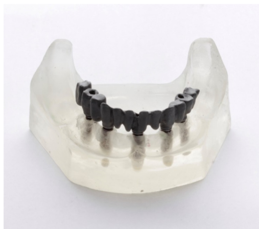
Fig. 3 Reference Co-Cr framework fabricated using additive manufacturing technology.
