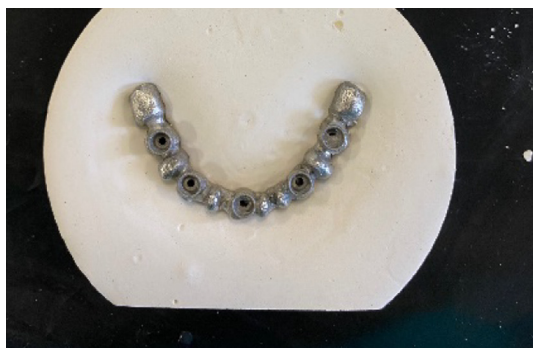
Fig. 6 Framework mounted to facilitate CMM measurement.
