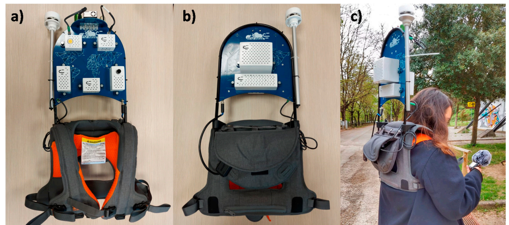
Figure 1. The new wearable system developed for monitoring outdoor environments: (a) front view; (b) back view; (c) system usage during a monitoring campaign.
