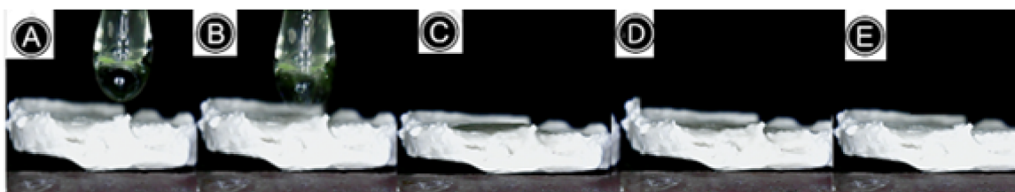
Fig. 9 Contact angles of PTBSA-SO 3 H: photograph of oil droplets.
