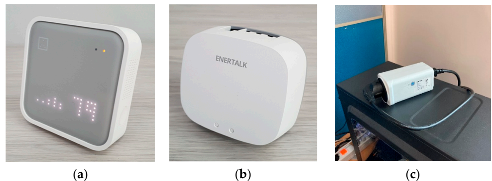
Figure 3. Environmental sensors (a) Awair Omni sensor, (b) Fuse box smart meter (Enertalk ENCORDED), (c) Individual household appliance smart meter (Enertalk Smart Plug).
