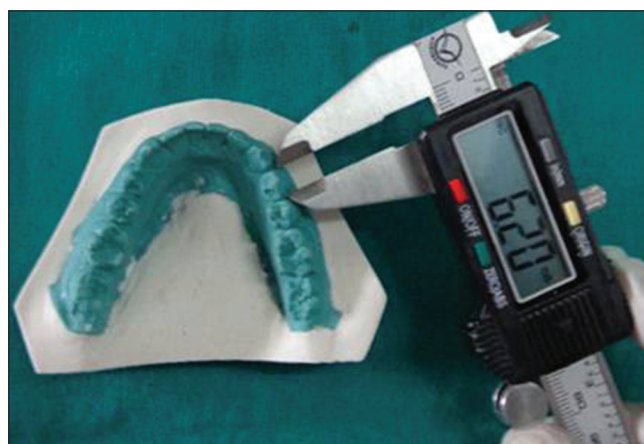
Figure 1: Measuring mesiodistal width using electronic digital calipers
