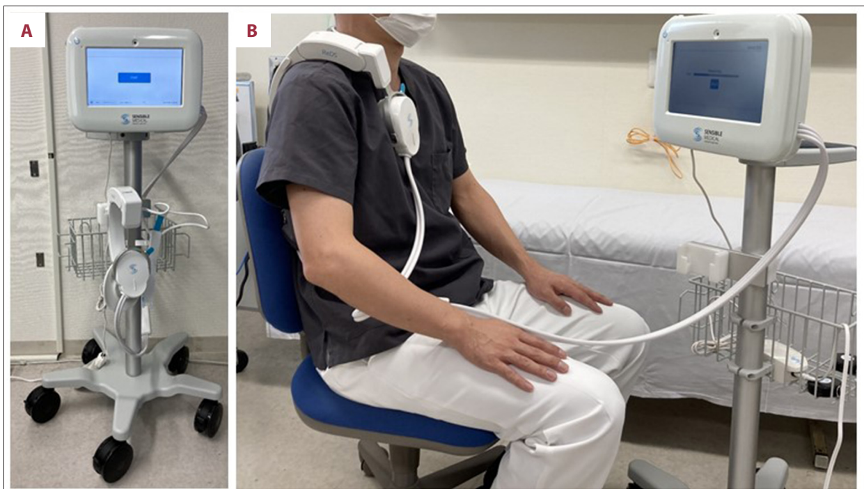
Figure 1. The remote dielectric sensing system: (A) a monitor (B) and a sensor.
