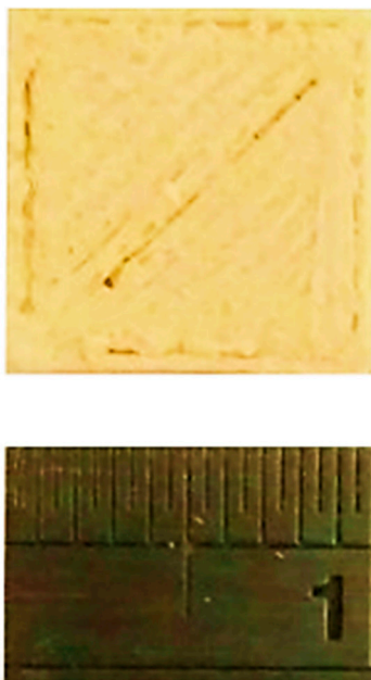
Figure 1. Typical photograph of a 3D-printed nanocomposite photocatalytic sample with 40% w/w TiO 2 in polystyrene (PS).
