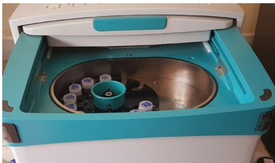
**Fig. 2.** Spectro Xepos spectrometer with a sample plate of 12 positions disposed of for EDXRF analysis. The first two positions on the plate are reserved for calibration samples and other positions for the samples under investigation.
