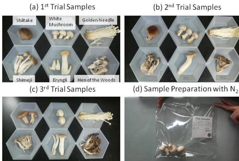
Figure 1. Approximately 30 g of mushrooms used for measurements (a)–(c) and the sample bag that was filled with dry nitrogen after placing the mushrooms inside (d).
