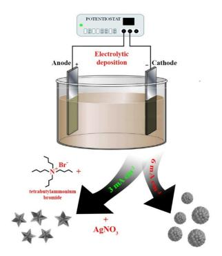
**Figure 1.** Schematic diagram of two methods for the synthesis of bimetallic Pd–Ag nanoparticles: "nanostar" and "nanoparticle".
