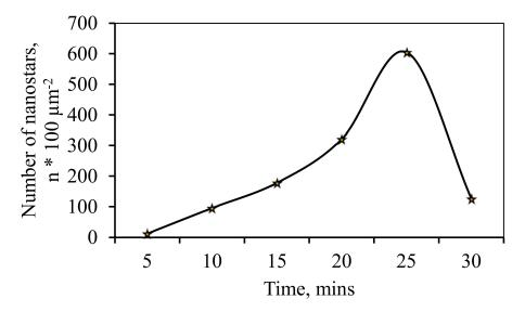
**Figure 7.** Graph of the dependence of the number of "nanostars" on the area of 100  $\mu$ m<sup>2</sup> on the time of film deposition.
