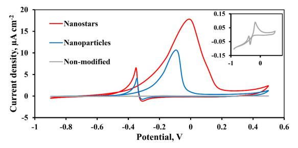
**Figure 11.** The cyclic voltammetric (CV) profile of steady cycles (30th) presented in current density in  $\mu$ A cm<sup>-2</sup> of the Pd-23%Ag electrode without a catalyst and of the Pd-23%Ag electrodes with "nanoparticle" and "nanostar" type catalysts for alkaline methanol oxidation in 0.5 M methanol in 1.0 M NaOH at room temperature with a scanning potential rate of 50 mV s<sup>-1</sup>.
