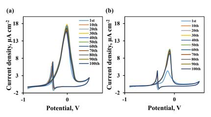
**Figure 12.** Multiscanning of Pd-23%Ag CV electrodes with "nanostar" (**a**) and "nanoparticle" (**b**) catalysts up to 100th cycle in 0.5 M methanol in 1 M NaOH at 50 mV s<sup>-1</sup> scan rate.
