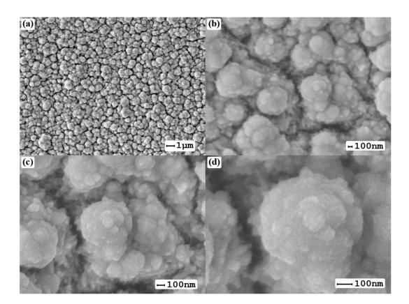
**Figure 3.** SEM images of the surface of palladium–silver films with a modified surface using the "nanoparticle" method at magnifications of 5000 (**a**), 30,000 (**b**), 50,000 (**c**) and 100,000 (**d**).
