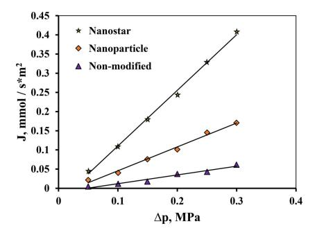
**Figure 14**. Dependence of the flux on the excess pressure of hydrogen at 25 °C on the input side of the unmodified Pd-23%Ag membrane and Pd-23%Ag membranes modified by the "nanoparticle" and "nanostar" methods.
