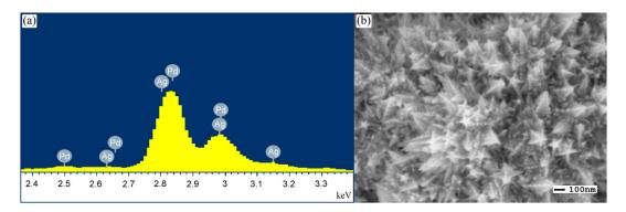
**Figure 10.** SEM image (**a**) and EDX spectra of Pd–Ag membrane samples modified by "nanostar" method (**b**).
