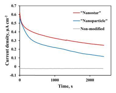
**Figure 13.** Chronoamperometric profiles for Pd-23%Ag electrodes without catalysts and for Pd-23%Ag electrodes with "nanoparticle" and "nanostar" catalysts for 0.5 M methanol in 1 M aqueous NaOH solution at potential of -0.3 V up to 2400 s.
