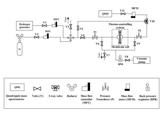
Figure 2. Diagram of the installation for measuring hydrogen permeability.
