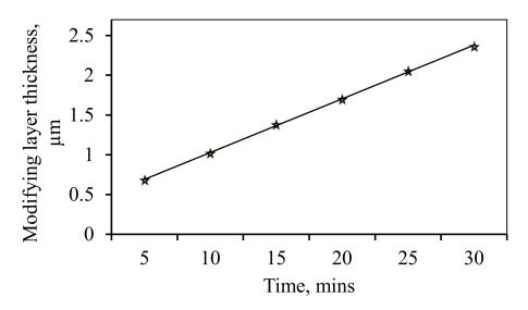
**Figure 6.** Graph of the dependence of the thickness of the modifying coating of the "nanostar" type on the time of film deposition.
