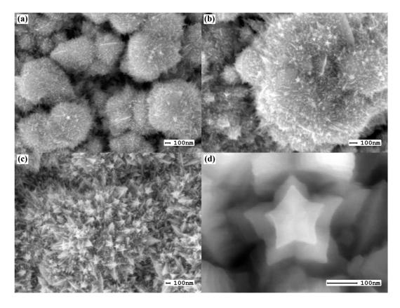
**Figure 5.** SEM images of the surface of Pd–Ag membranes modified by the "nanostar" method after electrolytic deposition for 5 min (**a**), 15 min (**b**) and 25 min (**c**,**d**).
