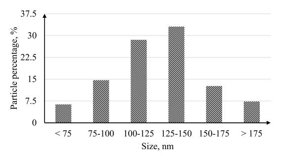
Figure 8. Histogram of the size distribution of nanoparticles obtained by the "nanostar" method.
