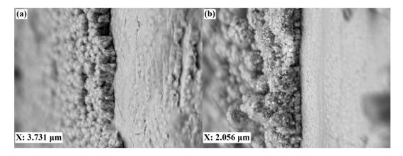
**Figure 9.** SEM images of sections of palladium–silver films modified by "nanoparticles" (**a**) and "nanostar" (**b**) methods.
