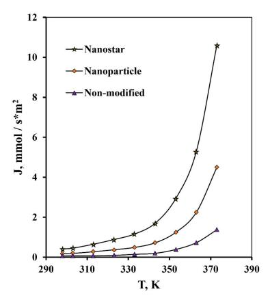
**Figure 15.** Temperature dependence of the hydrogen flux at  $\Delta p = 0.3$  MPa through a non-modified Pd-23%Ag membrane and Pd-23%Ag membranes modified by the "nanoparticle" and "nanostar" methods.
