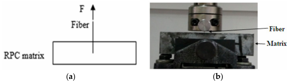
Figure 1. Single-fiber pull-out test: (a) schematic and (b) photo.
