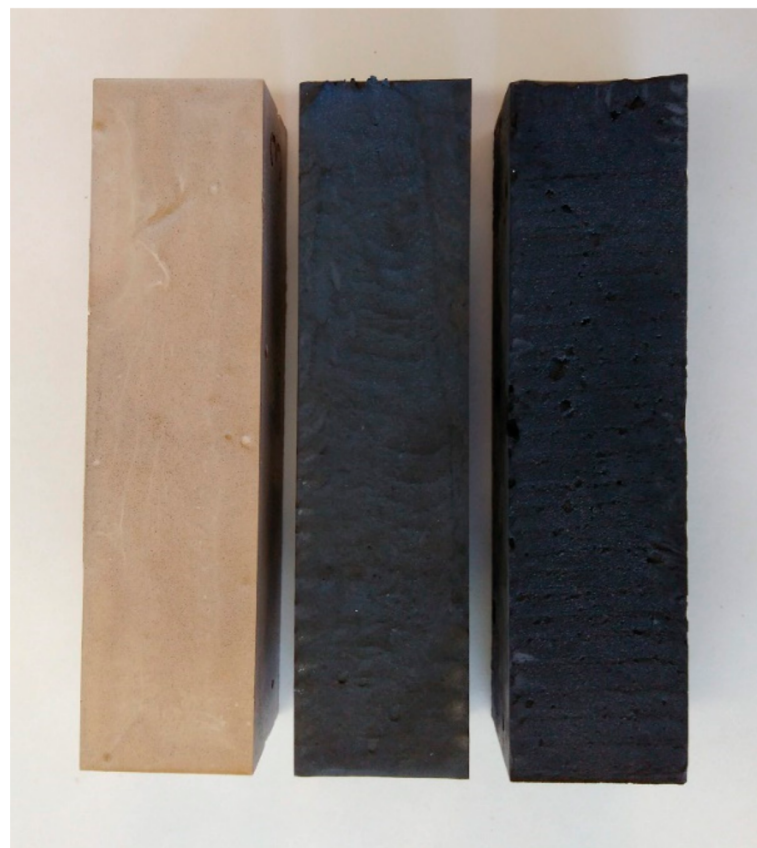
Figure 2. Photograph of the prepared composites MOC-CNT-R (left), MOC-CNT-0.5 (middle), and MOC-CNT-1 (right).
