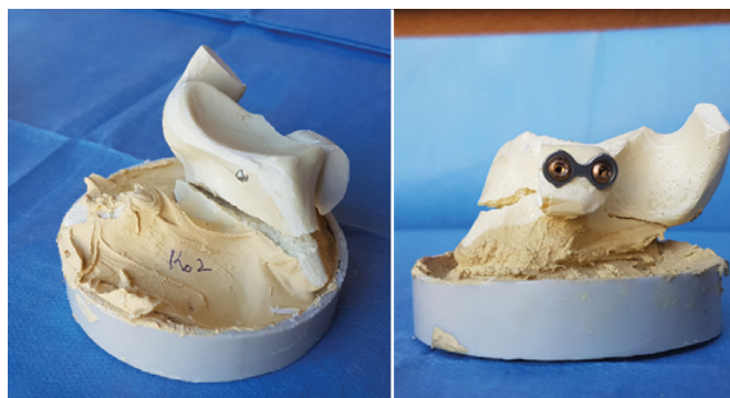
Figure 4. Glenoid neck fracture during the test.
