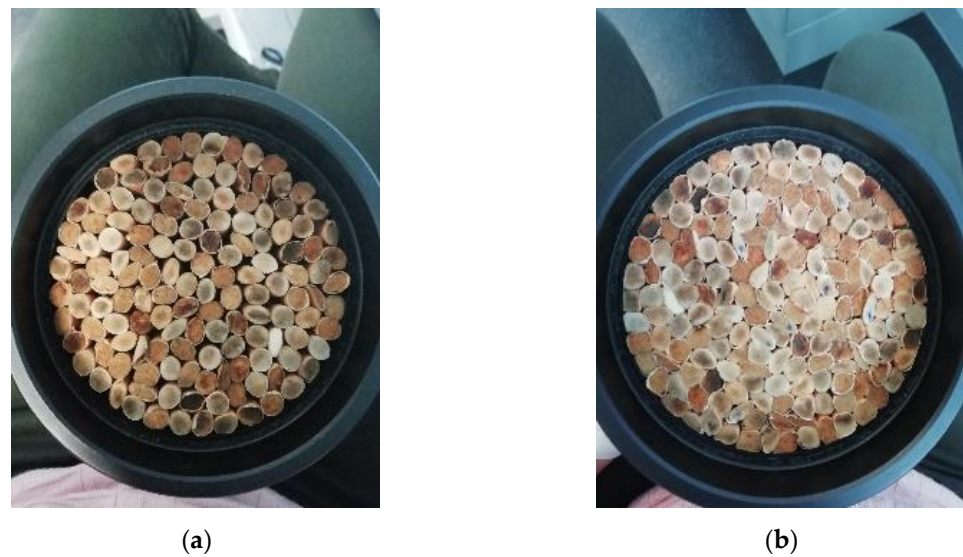
Figure 1. Example pictures of some of the prepared samples for the compaction study. Samples prepared with 140 (a) and 180 (b) used cigarette butts.
