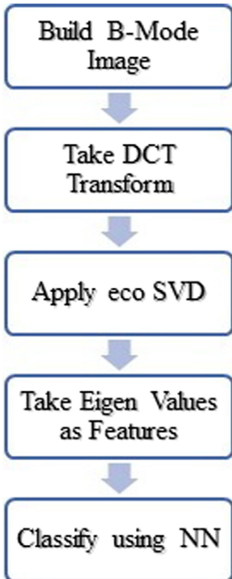
FIG. 4. Procedure scheme for sonogram classification.
