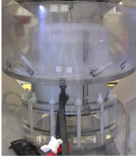
Fig. 1. The standard flotation vessel with external launder.
