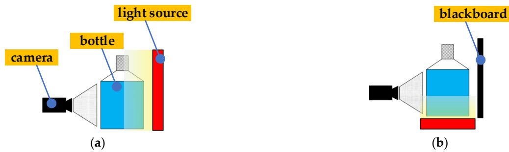
Figure 3. Black and white impurity lighting schemes. (a) Black impurity lighting scheme; (b) White impurity lighting scheme.
