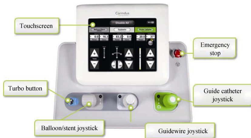
Figure 2. Control console components.
