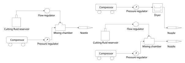
Figure 2. Schematics of MQL and MQCL systems.
