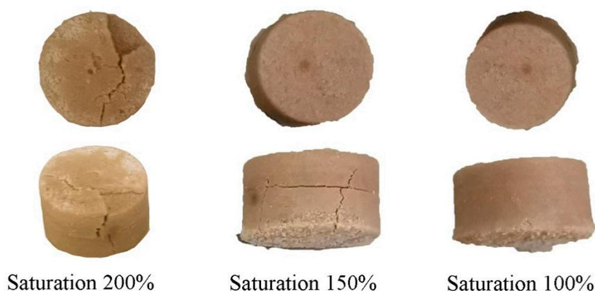
**Figure 7.** Images of F-BaTiO<sub>3</sub> samples printed by BJ with different saturation after sintering. Scale: each sample has a diameter of 15 mm and a height of 10 mm. Heating rate of 10 °C/min to 1400 °C with a dwell time of 4 h.
