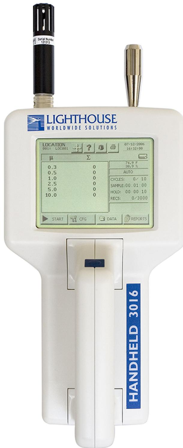
**Figure 1** Lighthouse 3016 particle counter.
