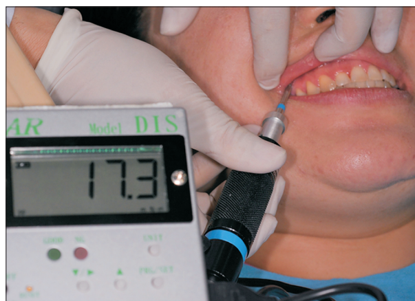
Figure 3. Measurement of the placement and removal torques by using a digital torque gauge.
