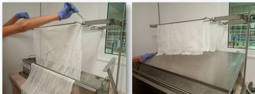
Figure 7. Homemade bath for nets' coating with antimicrobial polymers on a pilot scale, equipped with a drying hang and a stainless-steel inclined surface.
