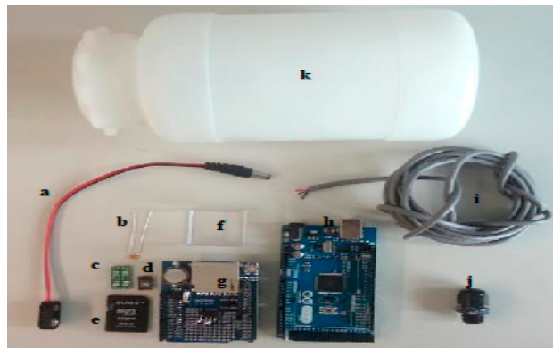
Figure 3. KdUINO components, (a) 9 V Battery button power plug for Arduino; (b) 100 nF Capacitor; (c) 8 pin SOIC to DIP8 Adapter; (d) SD memory card; (e) TSL230RP; (f) Polyester transparent box; (g) Data Logger Module Logging Recorder Shield V1.0; (h) Arduino MEGA 2560 R3; (i) Industrial cable, 3 cores; (j) Cable Gland Nylon 66; (k) Hermetic bottle.
