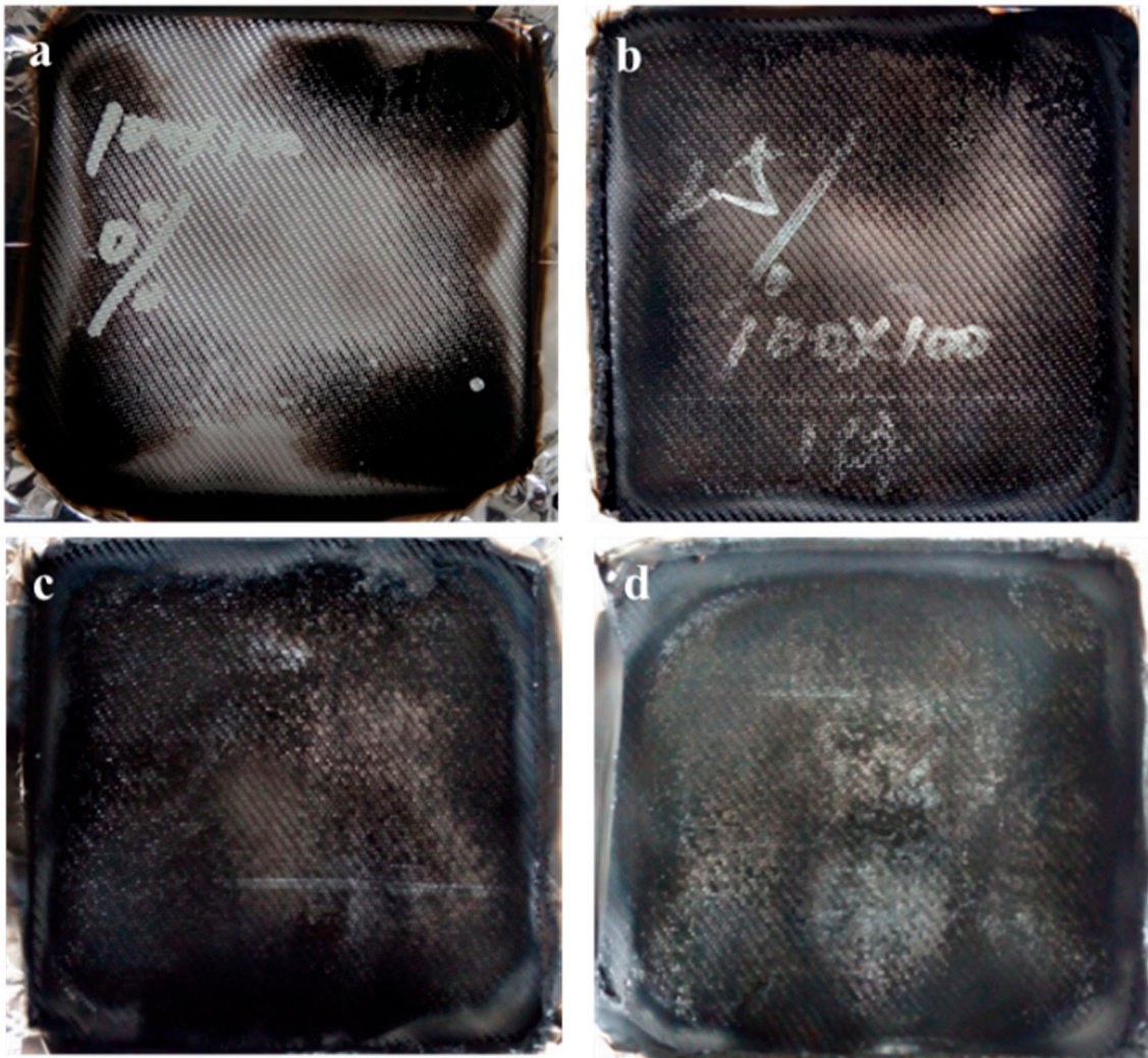
Figure 7. Digital pictures for RTM epoxy composites preformed by ET3228 tackifiers containing (a) 0, (b) 23, (c) 38 and (d) 48 wt.% MRP after the cone calorimeter test.
