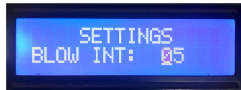
Fig. 26 Display with the Blow Intensity function set to the maximum intensity
