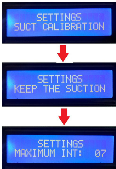
Fig. 20 Display with the Suction Calibration messages
