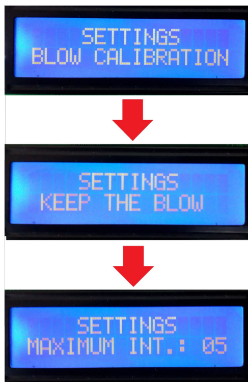
Fig. 19 Display with the Blow Calibration messages
