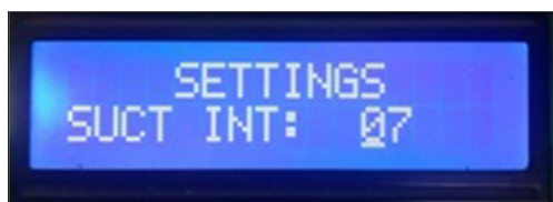
Fig. 27 Display with the Suction Intensity function set to the maximum intensity
