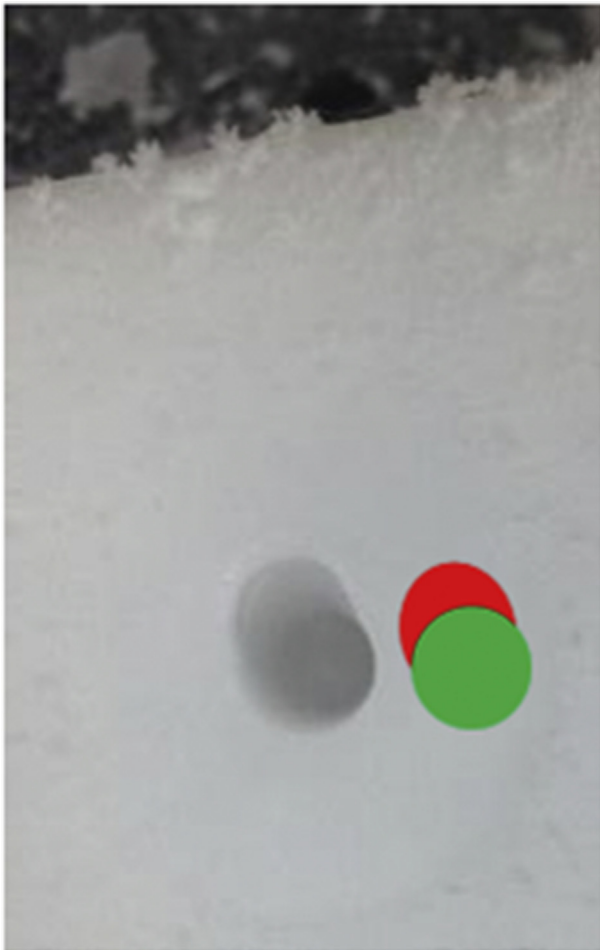
Figure 5. Oblong bore caused by lateral slipping of the pick. Visual aid with desired (green) and undesired (red) bore area.
