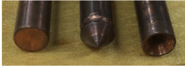
Figure 10. Flat, conical, and inverse conical tips shown left to right.
