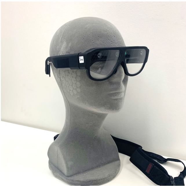
Figure 1. Generation 2 headset with mounted cameras for use with a left-sided 44-channel suprachoroidal retinal prosthesis (coils that connect to receiver–stimulators are not pictured). This component works in conjunction with an external processing unit or laboratory-based system.
