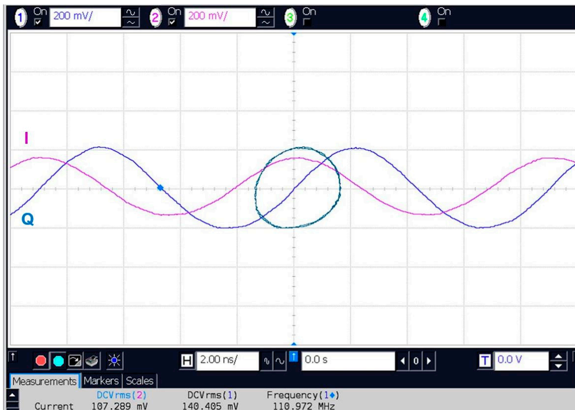
Figure 47. Quadrature baseband signals and the corresponding Lissajous graph.
