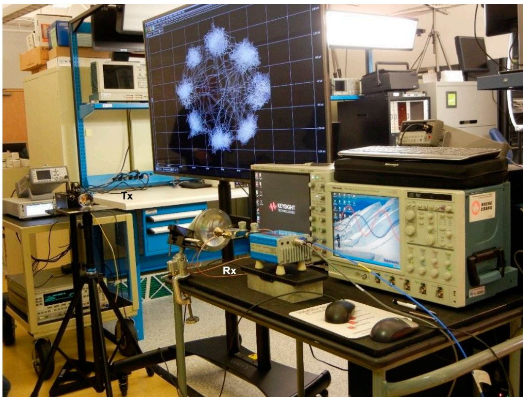
Figure 40. V-band multi-port characterization test-bench using modulated signals.
