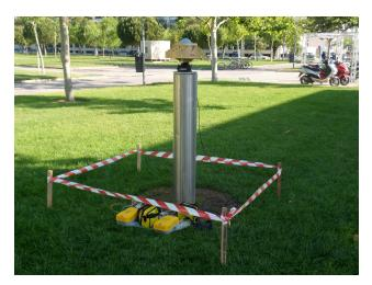
**Figure 1.** Global Navigation Satellite System (GNSS) measurement at the Universitat Politècnica de València (UPV) calibration baseline using a 3D choke-ring antenna equipped with a signal splitter and two receivers collecting the same signals.
