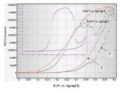
**Figure 10.** Influence of a scan rate of potential on electrochemical behavior (and cyclic polarization curve) of the Ti/PAAT/Ni electrode: 1—at a potential scanning rate 0.01 V/s (the first cycle). 2—at a potential scanning rate of 0.03 V/s (the first cycle). In the insert—at a scan rate of potential 0.1 V/s (the first cycle).
