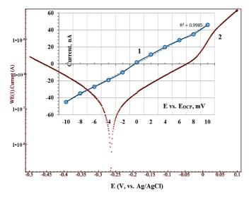
**Figure 7.** Linear sweep voltammogram of Ti/PAAT/Ni sample after stabilizing the free potential of corrosion (2). In the insert—a small part of this voltammogram within the potential range from -10 to 10 mV (curve 1).
