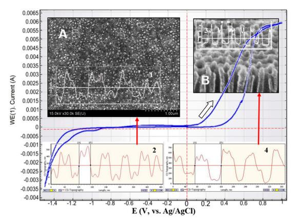
**Figure 8.** Cyclic voltammogram of the Ti/PAAT/Ni sample in the 0.9% aqueous solution of NaCl at a potential scanning rate of 0.1 V/s. In the insets: (A)—top view and AFM-profiles (1,2) of the experimental sample (NiNPs in PAAT) after alumina partial etching, (B)—cross-section views and AFM-profiles (3,4) of the experimental sample (PAAT) before NiNPs deposition into  $Al_2O_3$ .
