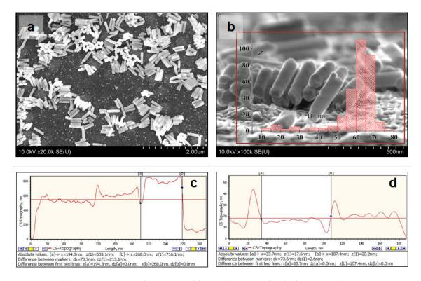
**Figure 2.** (**a**,**b**)—SEM images and histogram of the sample, obtained in dc-deposition of Ni at a constant potential -1.8 V within 5 min, after alumina selective chemical etching, (**c**,**d**)—AFM profiles of this sample surface for estimating the NPs diameter.
