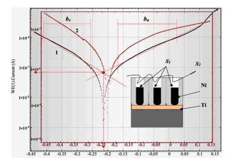
**Figure 6.** Linear sweep voltammograms of the Ti/PAAT/NiNPs sample in the 0.9% NaCl aqueous solution at a potential scanning rate of 0.1 V/s: 1—the fourth cycle of polarization, 2—the second cycle of polarization.
