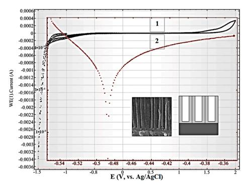
**Figure 4.** Cyclic (1) and linear sweep (2) voltammograms of the Si/SiO<sub>2</sub>/Ti sample in the 0.9% aqueous solution of NaCl at a potential scanning rate of 0.1 V/s.
