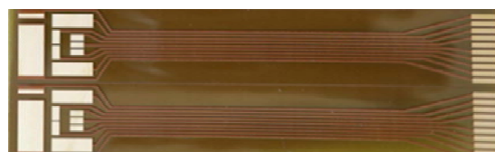
Figure 4. Two of the flexible designed electrodes systems dedicated to glucose measurements in sweat.
