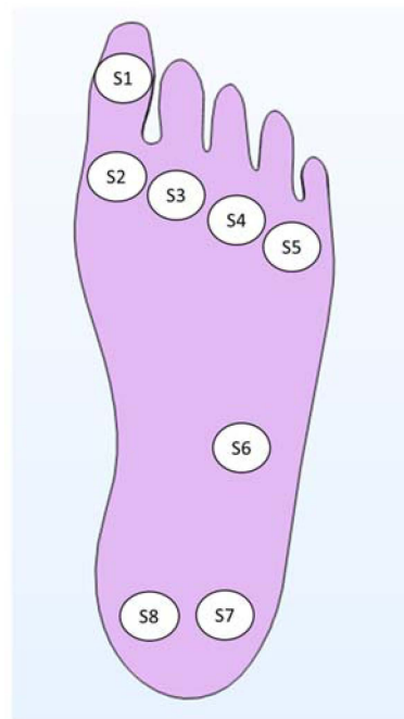
Figure 2. Eight sensing points distributed on the main foot points where impending subcutaneous tissue damage are likely to occur.
