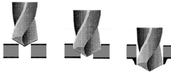
Figure 7. Burr formation when drilling using a pilot hole.
