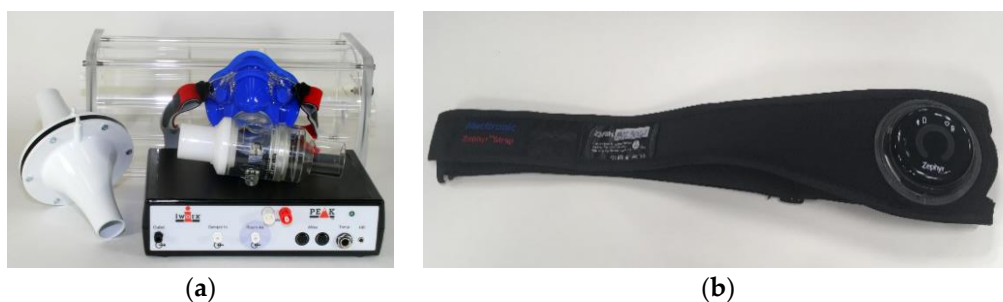
Figure 9. Respiratory technologies. (a) airflow, (b) strain gauge.
