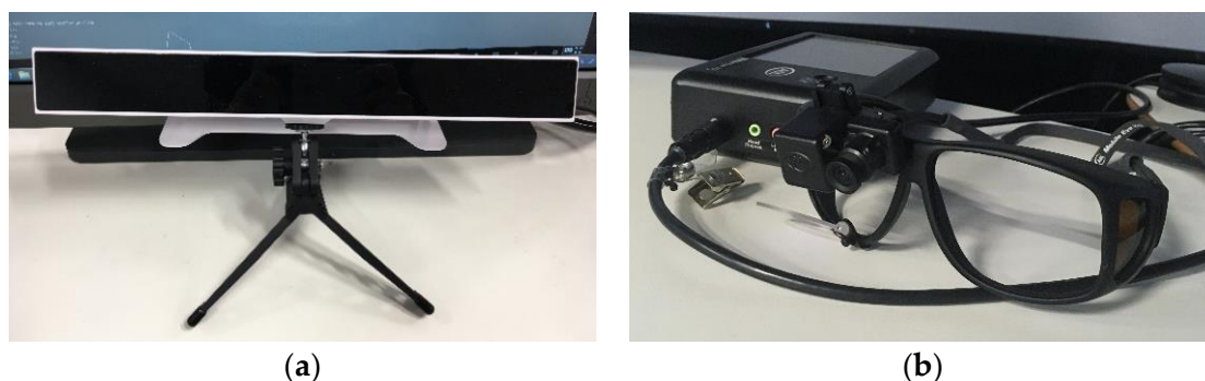
Figure 6. Eye tracking technologies used in HFE Lab . (a) remote sensor, (b) wearable sensor.
