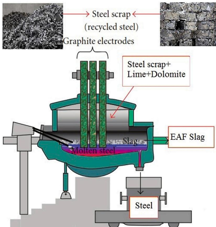
Fig. 1. The schematic drawing of EAF steelmaking process.
