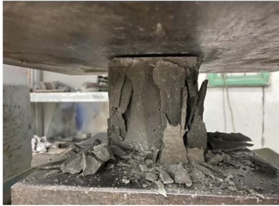
(a) Compression failure in ordinary cement binder after freeze–thaw cycles
