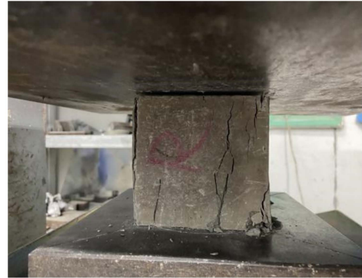
(b) Compression failure in polymer-modified cement binder after freeze–thaw cycles
