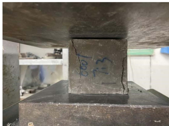
(c) Compression failure in 30% P1-blended cement binder after freeze–thaw cycles
