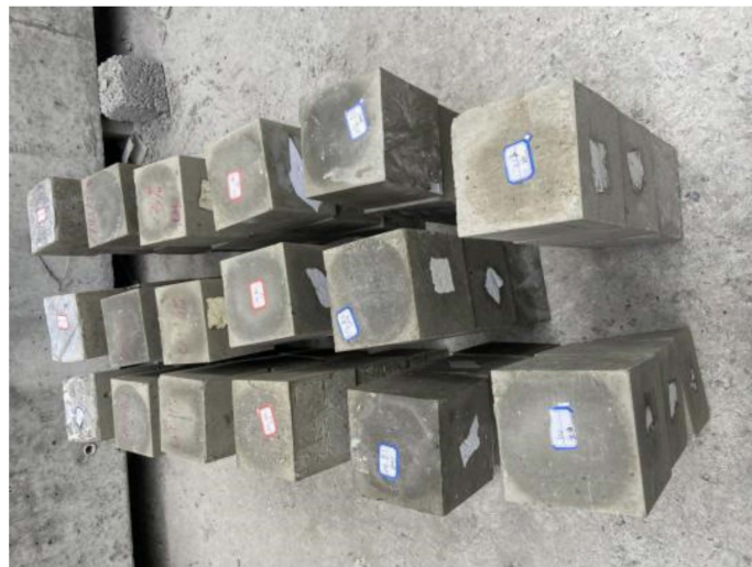
Figure 4. Test specimen for freeze thaw.
