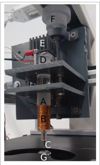
FIGURE 2 | Setup of the illuminated electromagnet. Acrylic pole (A), copper coil (B), iron rod (C), LED-chip (D), heatsink (E), vertical positioning mechanism (F), objective of the microscope (G).
