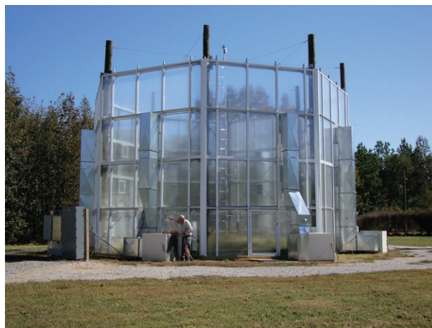
Fig. 1. A prototype warming chamber constructed at Oak Ridge National Laboratory that is being tested for refinement before deployment for an ecosystem manipulation experiment in a spruce – peat bog near Grand Rapids, MN, USA ( https://mnspruce.ornl.gov/ ). Photo compliments of Paul Hanson, Oak Ridge National Laboratory.
