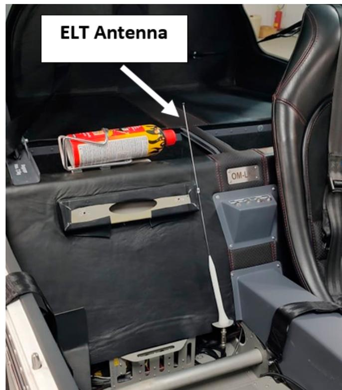
**Figure 2.** Location of the ELT antenna in a Tomark Aero s.r.o. Viper SD-4 RTC aircraft.
