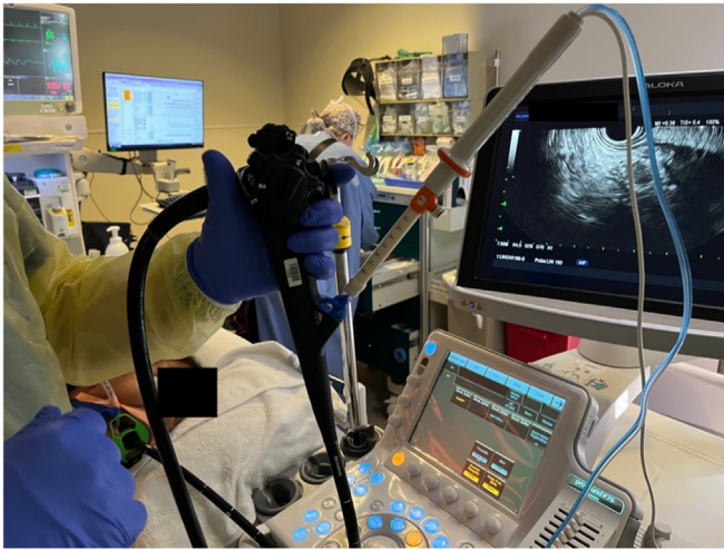
Figure 2. EUS-guided radiofrequency ablation device and setup. The 19-gauge trocar has been introduced into a linear echoendoscope. Catheters are seen connecting to the trocar to provide circulation of cold saline to prevent overheating of the device tip. EUS is used to locate the pancreatic mass and to guide the delivery of the radiofrequency energy.
