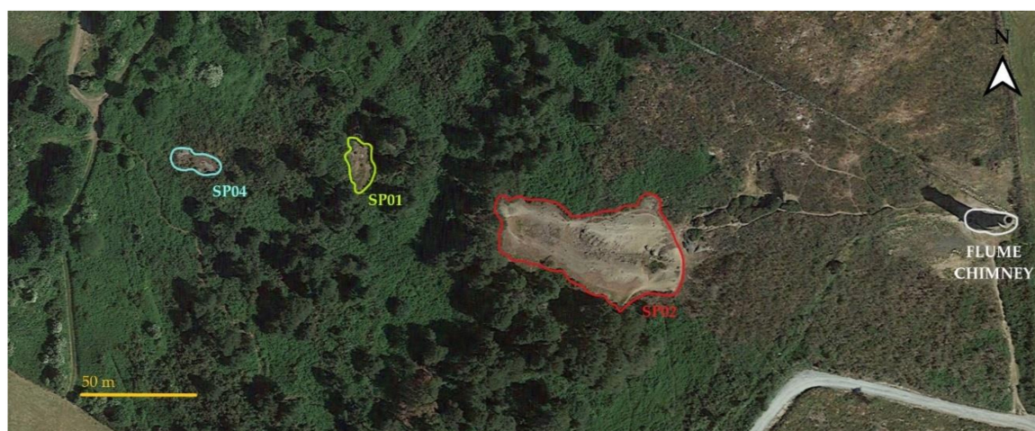
Figure 2. Ballycorus site map and spoil heaps (SP02, SP01, SP04). The flume chimney (highlighted in white) was the mine shaft site and was constructed in the early 1860s to vent the smelter smoke. SP02 was the original site used for lead ore and solid waste produced by these excavations are still accumulated at the edge of the heap representing the main volume of exposed mine waste. SP01 and SP04 are smaller solid waste heaps [23].
