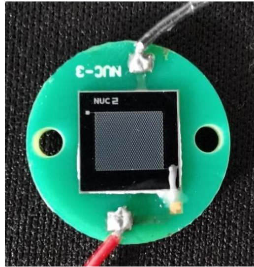
Figure 4. Photograph of the CMUT glued and wire-bonded to the printed circuit board (PCB).
