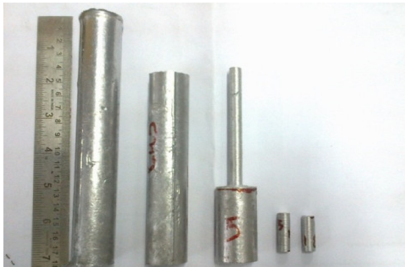
Figure 1. Illustrating the cast samples of the developed metal matrix composite (MMC).
