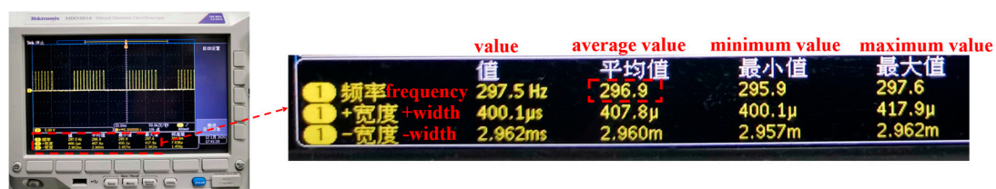
Figure 9. Pulse frequency captured by oscilloscope
