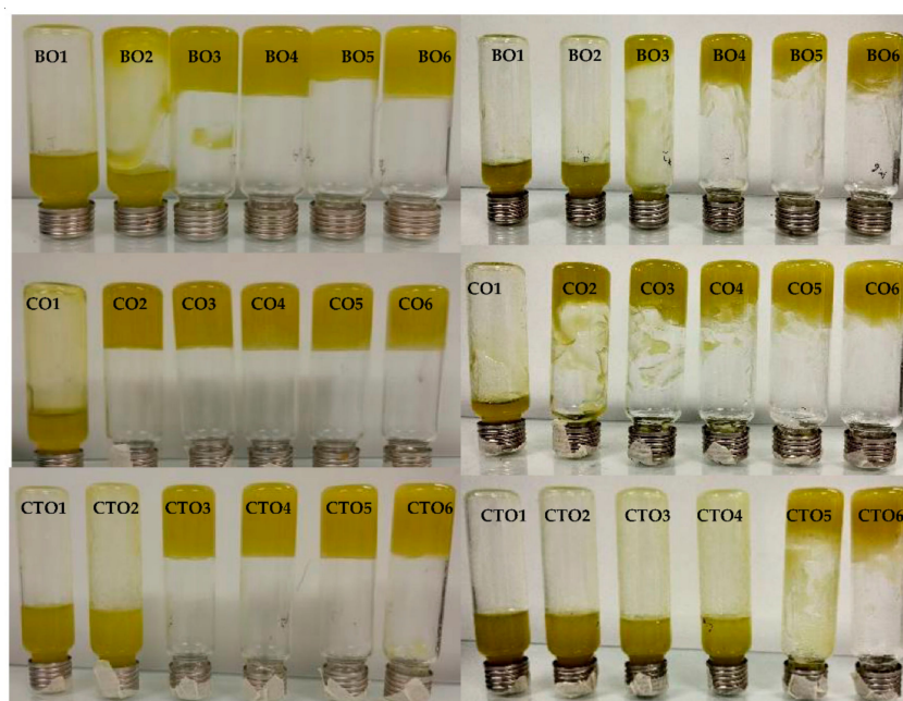
Figure 1. Inversion tests for beeswax ( top ), candelilla ( middle ) and carnauba ( bottom ) organogels. Samples are shown after production ( left ) and after two months of storage ( right ).
