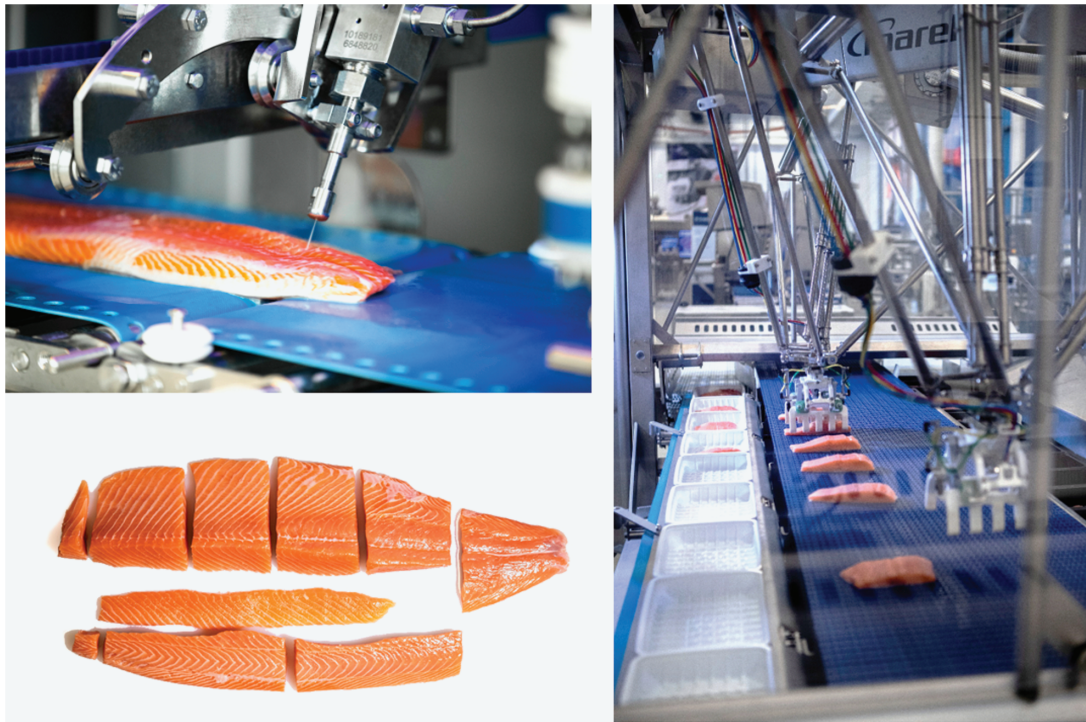
Figure 4. Salmon fillet processing. The pin bones of the fillet are removed with a guided robotic water jet cutter and portioned (top- and lower left pictures) and then picked by an automated gripper off the conveyor and placed into boxes. Courtesy of Marel.
