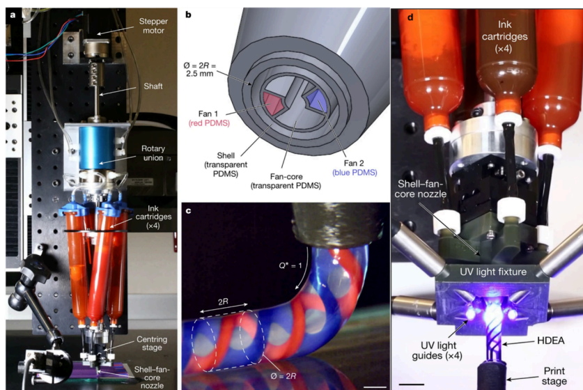
Figure 6. Rotational multimaterial printing with modified nozzle designs up to sub voxel control. Adapted from ref 53 with permission. Copyright 2023, Springer Nature Group.
